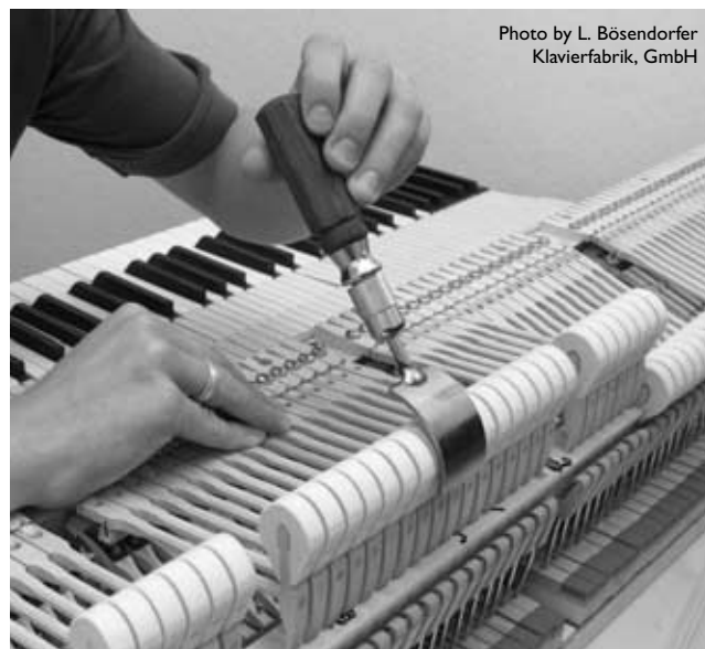
Figure 379 Ironing the hammers with a hand iron made by Meyne Klaviertechnik.
