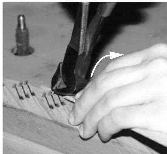
**Figure 442** Removing bridge pins with flush-cutting wire nippers. Note the wood strip that provides leverage and protects the bridge cap. Pull each pin in several short strokes.
