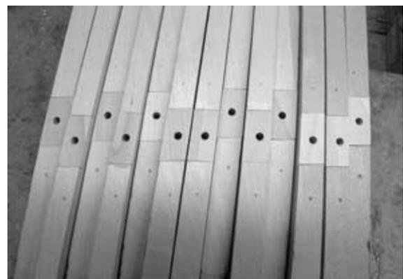
**Figure 417** Repairing elongated balance holes with hardwood blocks.
