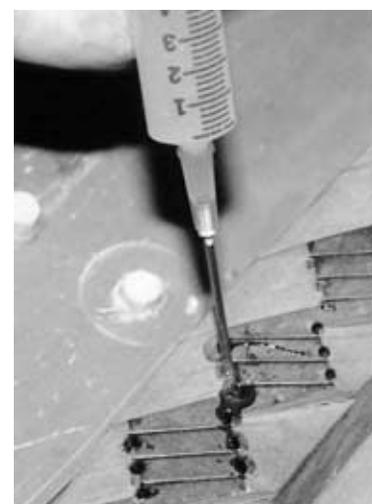
**Figure 443** Filling bridge pin holes with epoxy.
