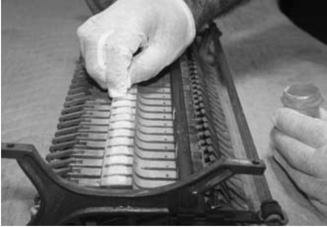
Figure 285 Applying and rubbing powder lubricant into wippen heel felts with a cotton glove.
