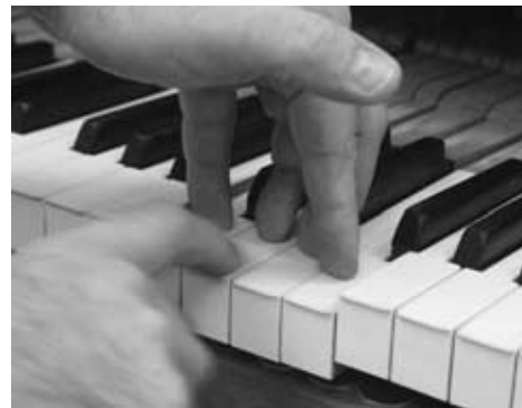
Figure 318 Testing whether the start of the bump on adjacent keys is level.
