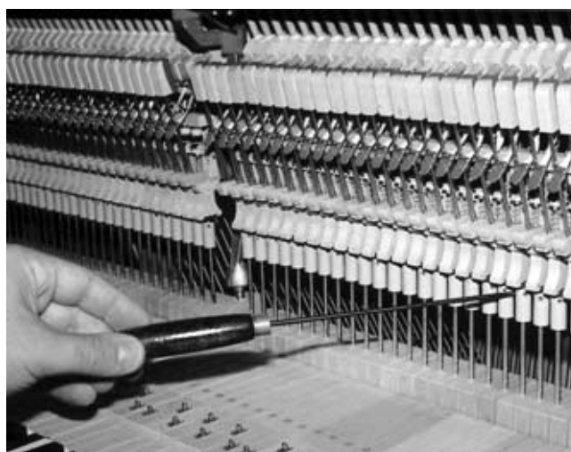
Figure 347 Adjusting the jack-to-hammer-butt gap by turning key capstans.
