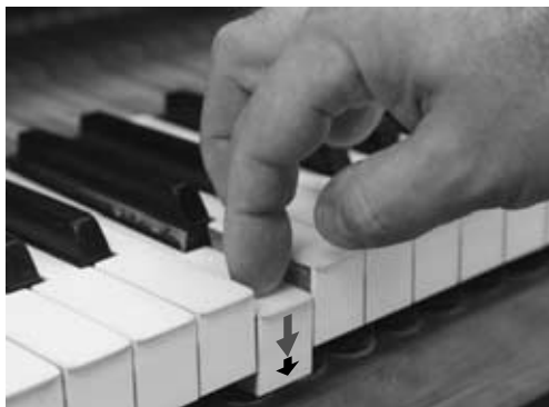
Figure 317 Testing the consistency of let off by playing off the jack.
