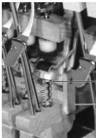
Figure 338 The jack spring should be positioned in wippen and jack notches, and the jack base must be firmly attached to the wippen.
