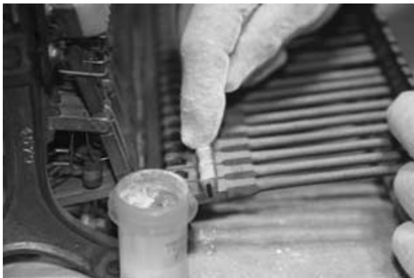
Figure 284 Rubbing a powder lubricant onto the knuckles with the top stack tilted forward.
