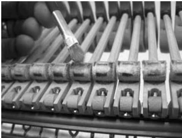
Figure 283 Applying powder lubricant with a cosmetics brush.
