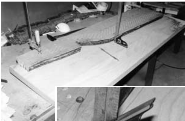
Figure 686 Marking the outline of the pinblock flange on the new plank.
