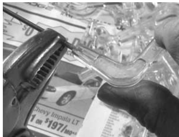
Figure 623 Winding a new elbow onto a sticker.
