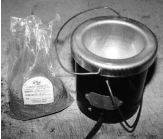
Figure 493 Hot hide glue and a thermostatically controlled pot.
