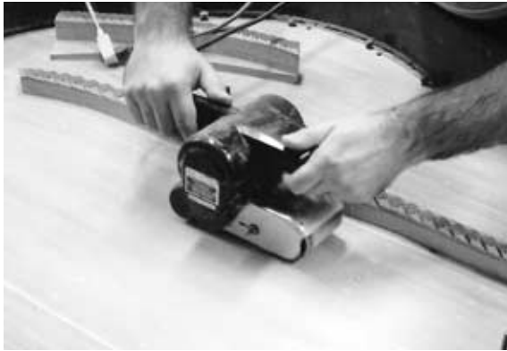
Figure 737 Sanding the soundboard with a belt sander.
