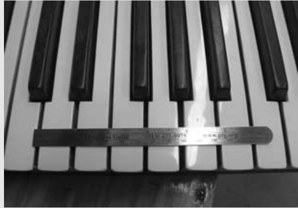
Figure 527 Overtrimmed keys can be widened by gluing a softwood veneer to their sides.
