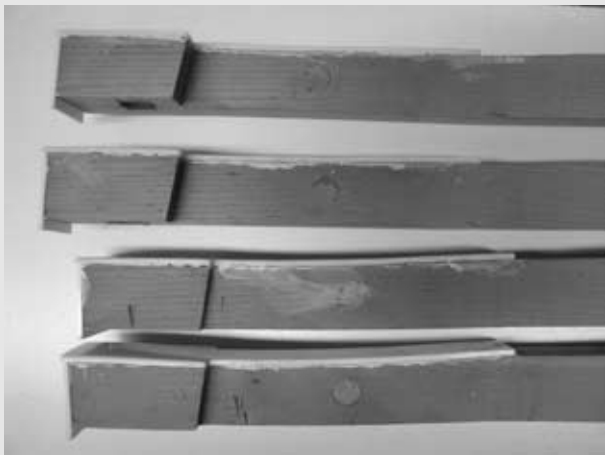
Figure 526 A poor key top replacement job like this one makes recovering the keys a challenge.
