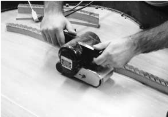
Figure 737 Sanding the soundboard with a belt sander.
