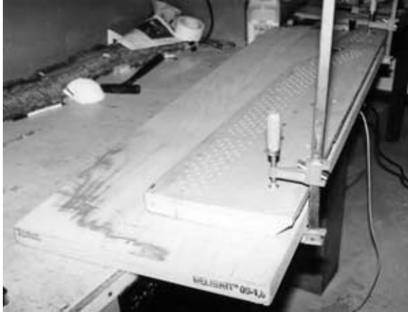
Figure 684 New plank ready for marking the outline of the original pinblock.
