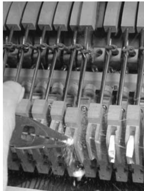
Figure 622 Crushing the remnants of old elbows.
