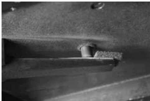
Figure 620 Bushed pitman dowel in a 1923 Steinway A III.
