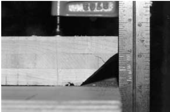
Figure 685 Aligning the old block (top) to the new plank (bottom) with a ruler. Note the small horizontal gap between the old block and the ruler.
