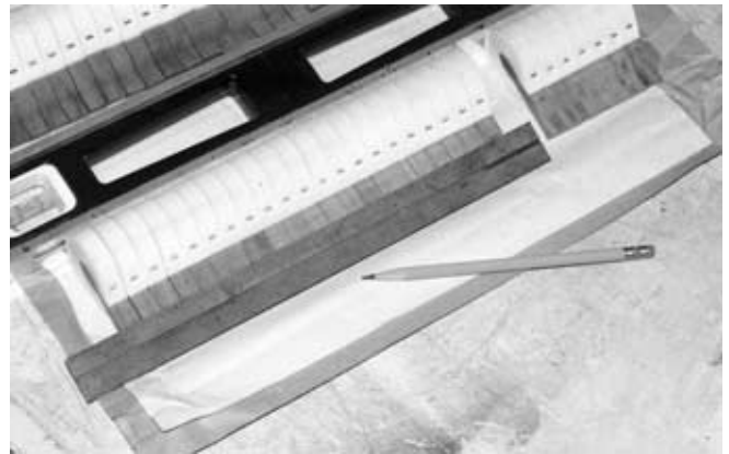
Figure 583 Marking the drilling positions on hammer moldings.
