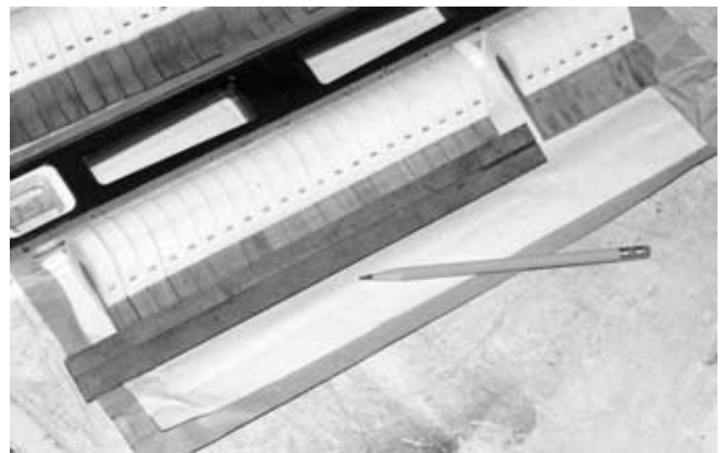
Figure 583 Marking the drilling positions on hammer moldings.
