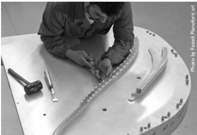
**Figure 108** Bridges are notched sideways at the Fazioli factory.
