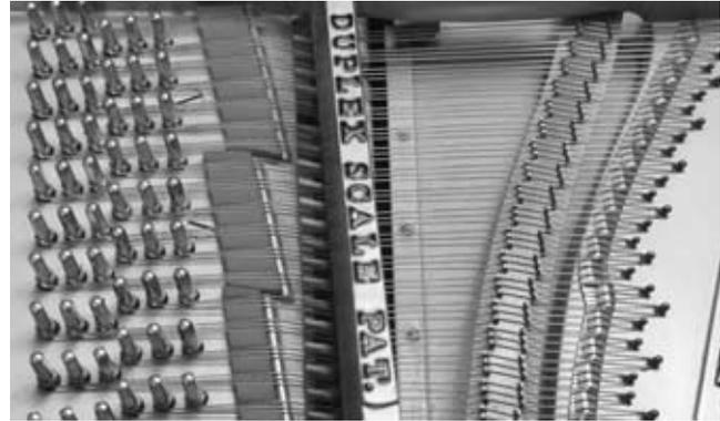
Figure 86 Front and rear duplex scales.
