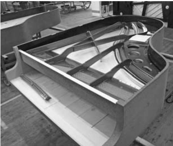
**Figure 31** Installed grand soundboard with bridges (top) and plate (bottom) (Bösendorfer factory).
